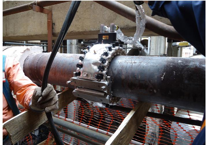
An 8" diesel line operating at 240°C (or 464°F) being tested by a HT inflatable ring.
