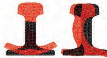
Example of guided wave mode shapes with energy concentrated in the foot (left) and web (right) of the rail respectively.
