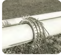
Transducer ring, early site test (circa 1994)
